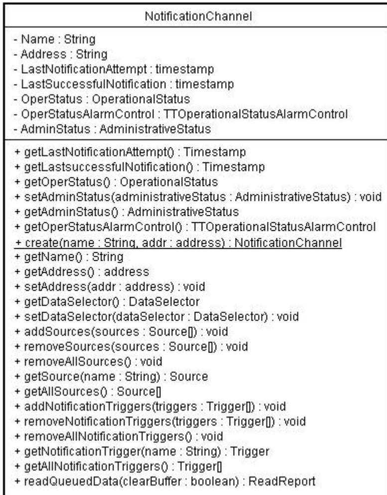
454 Figure 11 NotificationChannel Object UML
