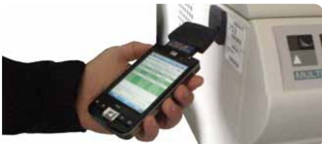
Personal Digital Assistant (PDA) with an attachable UHF reader
