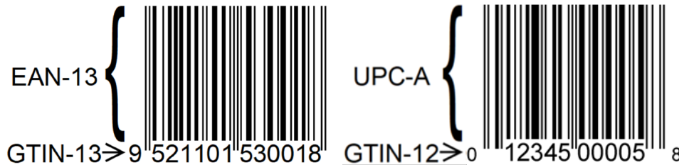
332 Figure 4-1 EAN-13 and UPC-A
