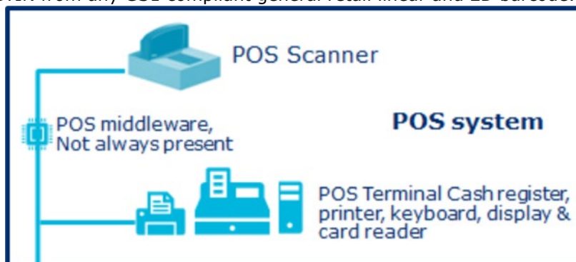
Figure 7-18 POS system with middleware feature
