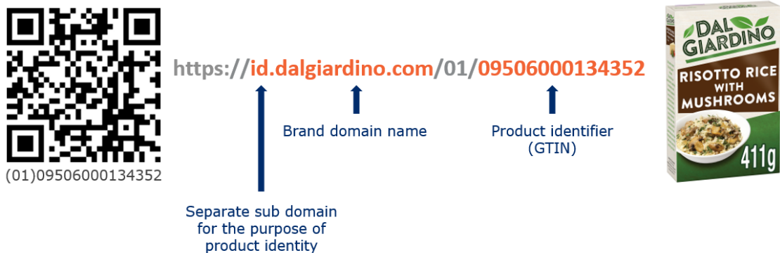
Figure 5-2 QR Code with GS1 Digital Link URI
