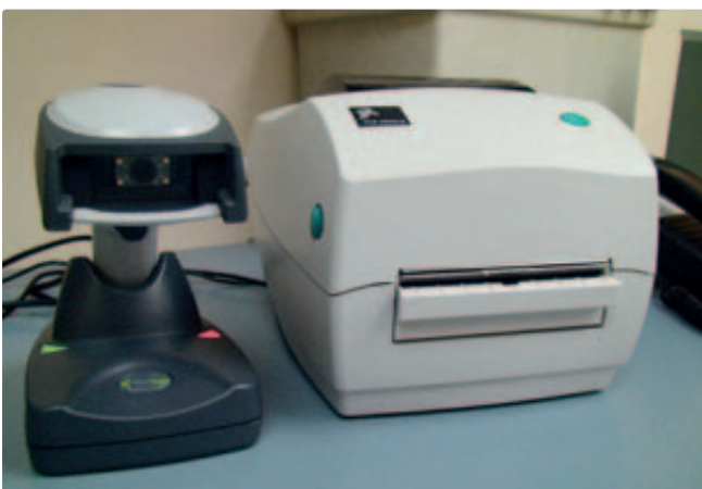
Bar coding station, including test scanner
