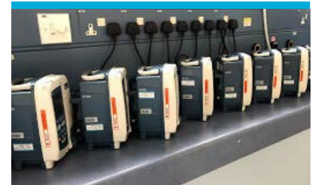
Figure 3: UHF passive tags used on infusion pumps for tracking
