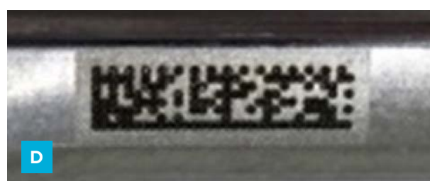
GS1 Datamatrix laser-engraved on a steel instrument C: 2,5 mm. D: 1,3 x 5,0 mm
