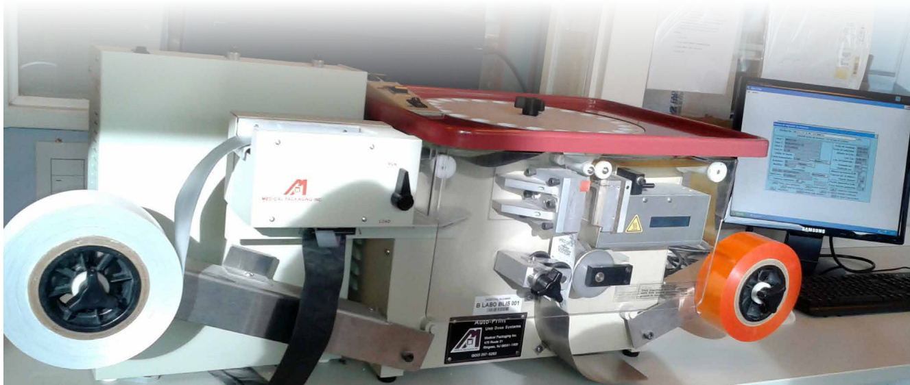
Figure 2: Machine for unit dose repackaging in the HA-Pharmacy
