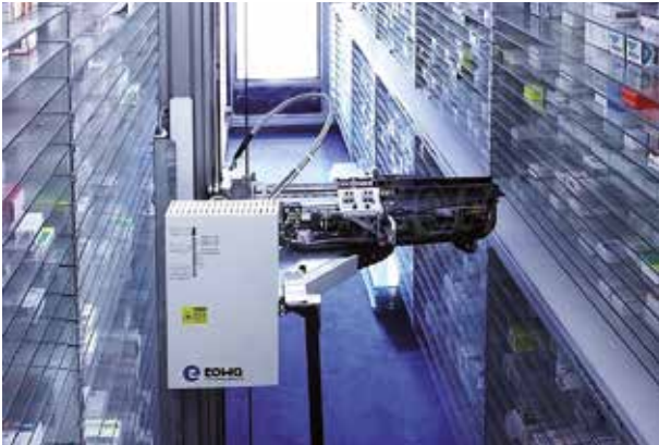
Picture 3 Internal structure of automatic integrated closed medicine cabinet
