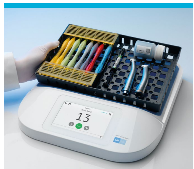
Instruments are uniquely identified with a GS1 Global Trade Item Number and serial number—identification data that is encoded as a so-called Serialised Global Trade Item Number (SGTIN) - in an EPC/RFID tag and can be read via wireless ultra high frequency (UHF) readers.
