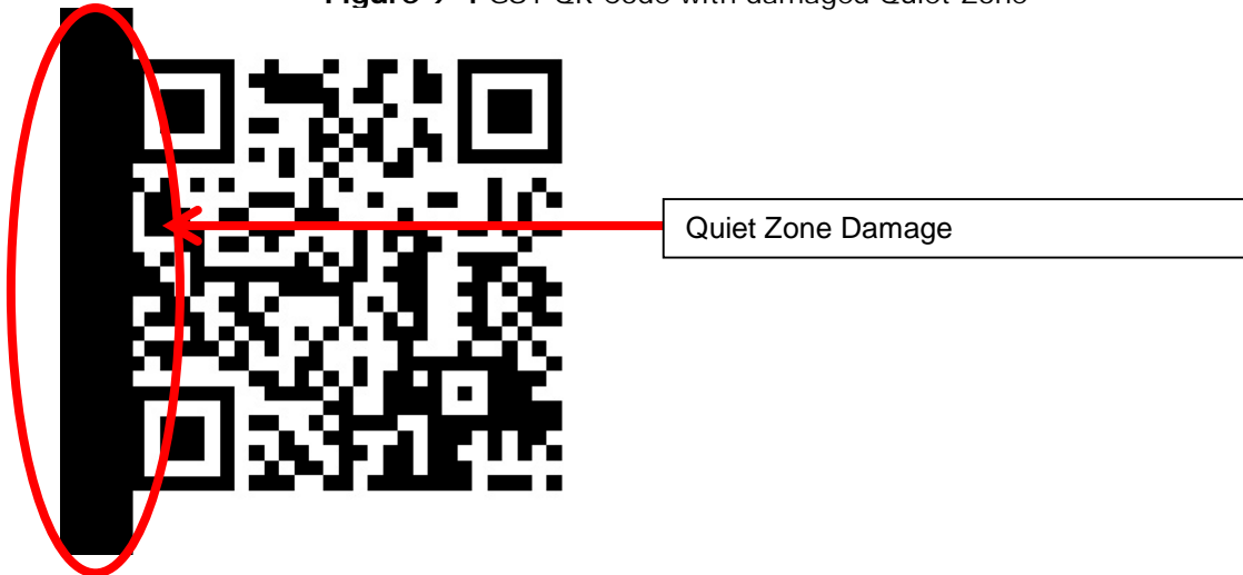
Figure 9-4 GS1 QR Code with damaged Quiet Zone
