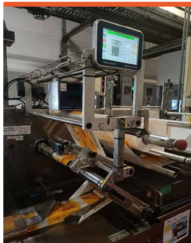
Thermal transfer printer, in Capriata d'Orba plant
